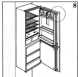
Position the furniture door runners B at the top and bottom of the door as shown in Fig. 9 (lining them up with the appliance door runners A), and secure them loosely. Experiment with the position of the furniture door runners, by sliding to the left or right until the doors run smoothly together. Tighten the furniture door runners and fit the snap-on covers C.
